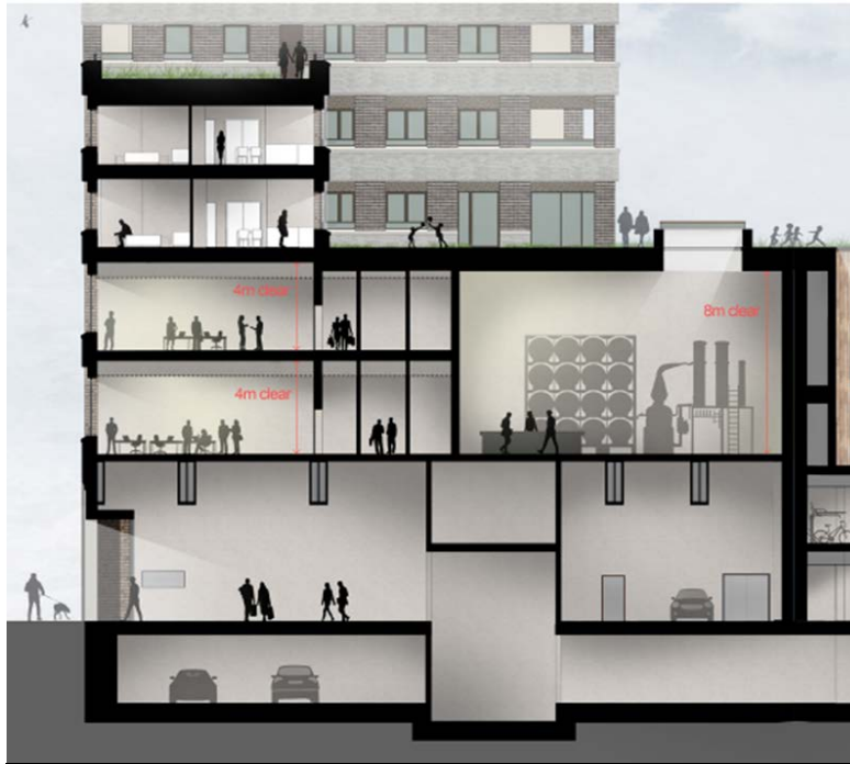
Image: Section showing floor to ceiling heights for B class floor space
